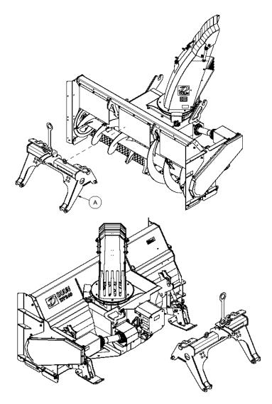
To use snow blower for front mounting or when reversing, the snow blower must change the direction of travel. Changing the direction of travel is done by turning three-point linkage to the opposite side of the snow blower. Loosen up two screws that hold the tree point linkage and use the tractor to turn it around on the opposite side. Remember to put screws back and secure them.
