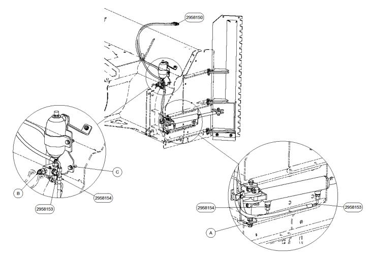
A: The bracket for cylinder must be mounted as in the illustration.
