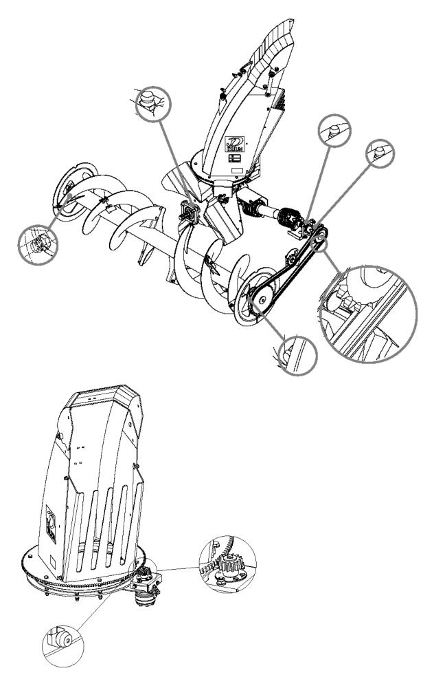
Before cleaning, lubricating, repairing or adjusting the machine, stop the engine and activate the handbrake, and remove the key during work. Close the safety crane on the snow blower that closes the oil on the operation of the feeder screw.
