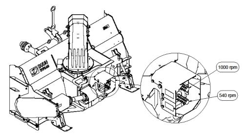
The snow blower is prepared for reversing and front mounting. The top pin marked with 1000 rpm is for a front drive. The bottom pin marked with 540 rpm is for reversing.
